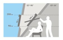
Centre-pivot roof windows make it possible to place furniture directly below the window without obstructing operation of the window.
